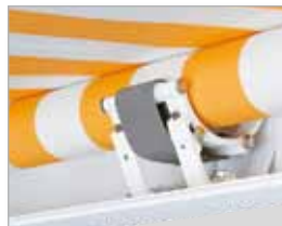
larger units are fitted with a rolltex bearing to prevent deflection of the roller tube
